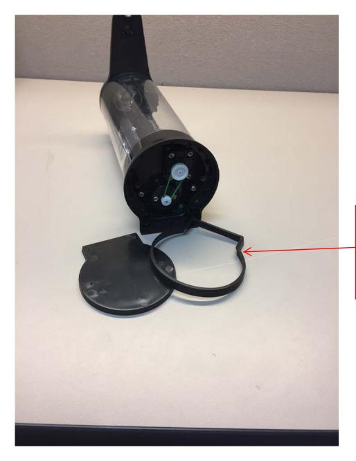
There is also a gasket located in the base to keep the dispenser water resistant. Make sure you replace it.
