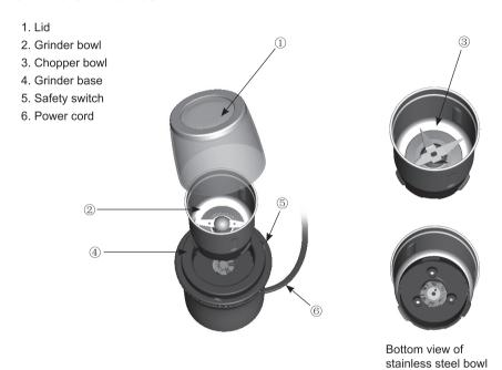
Grinder bowl is designed for grinding coffee bean and milling spices.
